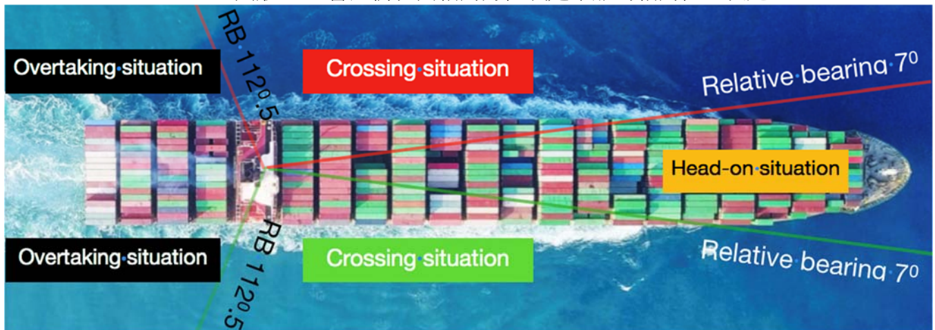
Figure 2-21 MEETING SITUATION BY RB OR RELATIVE POSITION OF TARGET VESSEL
